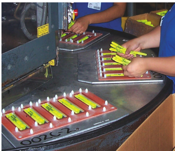
Blister-cavity platforms on Sanford's carousel heat-sealers accept the thermoformed blisters from a magazine. Workers then load the pens and apply backing cards before sealing.
