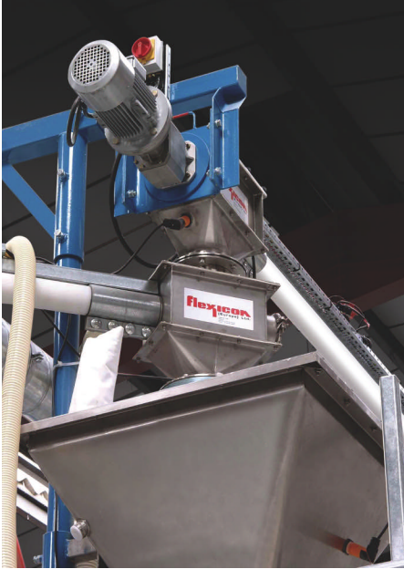
The first of three transfer points, a slide valve between the flexible screw conveyor and the hopper inlet opens and closes to regulate product flow.
